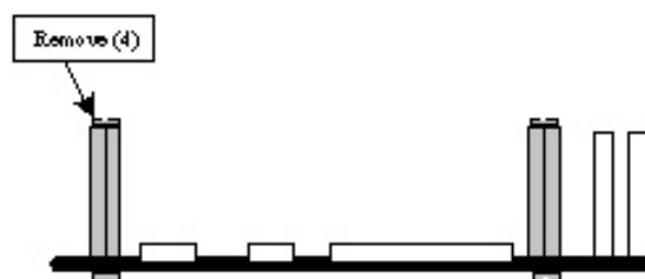
Figure 8-2 Remove four screws from exposed end
